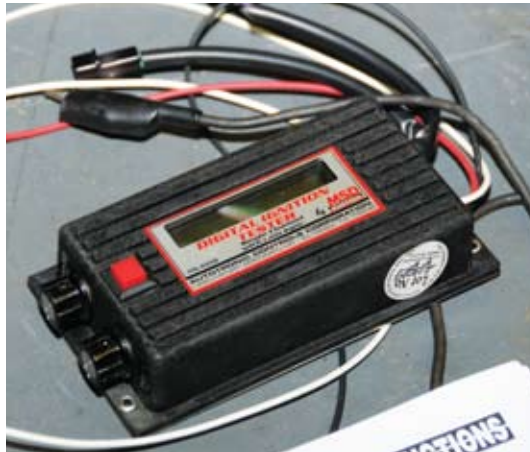
Once we installed the Power Grid system we chose to test fire it using MSD's Digital Ignition Tester.
