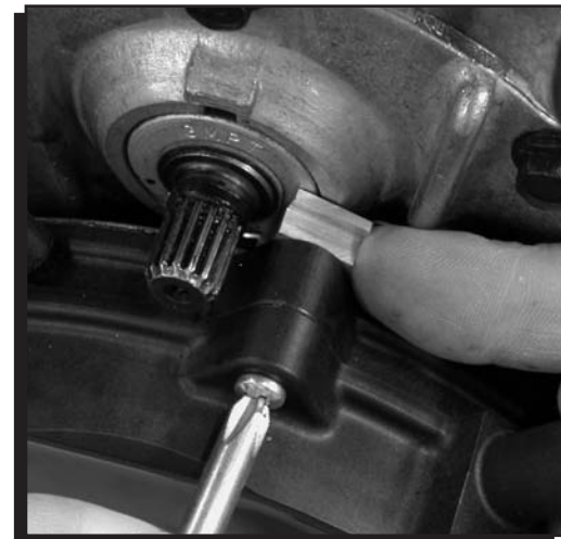
Figure 5 Clamp-Block Mounting Boss.
