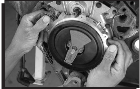
Figure 9 Installing the New Distributor.
