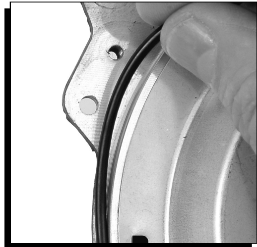
Figure 2 Installing the Distributor-to-Isolator Seal.
