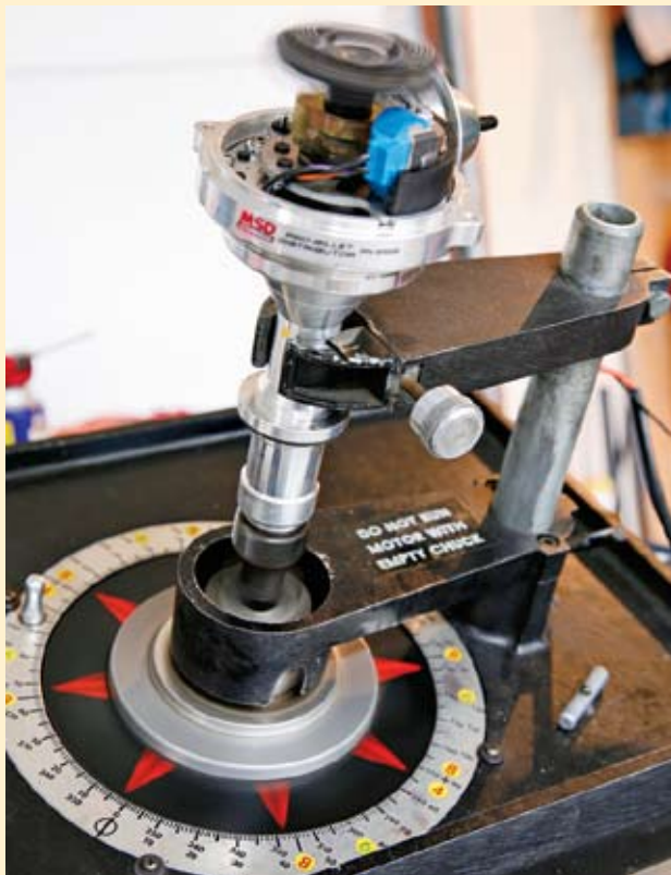
We checked the curve of the new MSD on the Allen syncrograph and found the factory curve to be spot on, then followed the instructions to change the total amount of mechanical advance and the rate of advance with the included bushings and springs. We checked the distributor again with the new components, and the curve matched the example graph in the instructions perfectly. This allows the end user to fine-tune the advance curve without a syncrograph.
