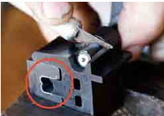
5 MSD has freed the weekend mechanic from having to buy a special ignition wire crimping tool with the addition of this ingenious two-piece fixture. It has a guide for measuring and cutting the insulator on the end of the wire and a die (red circle) for positive crimping of the connector to the wire.
