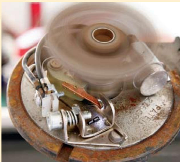
A close look at the original distributor at high speed revealed some pronounced point sparking. This is a result of point bounce and a tired capacitor.
