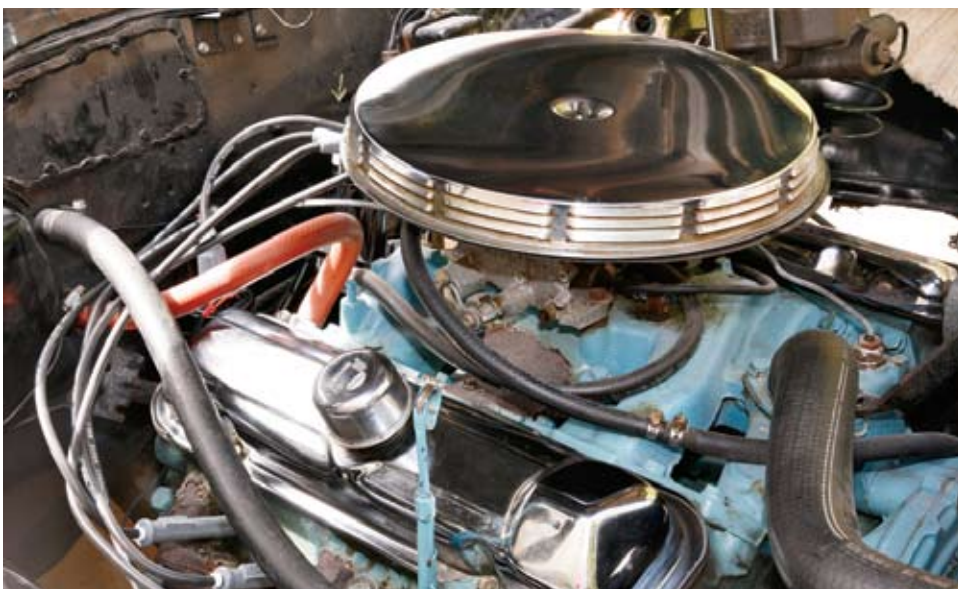
7 Connecting the MSD Pro-Billet distributor is as simple as connecting four wires. The red (switched 12V positive), orange (negative side of the coil), and black (ground) are grouped into one waterproof connector. The single gray wire is for the tach; it's also the wire used to program the internal rev limiter.
