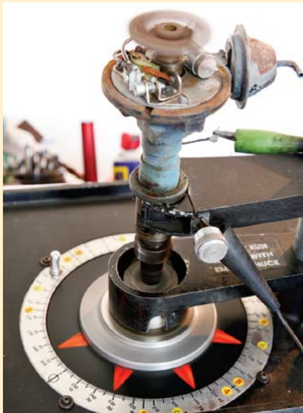
We were interested in seeing how the old GTO's original single-point distributor measured up on the Allen syncrograph. At 2,000 rpm (what would be 4,000-rpm crank speed) the strobes became erratic, as there should be eight solid triangles of red light around the base. This is the same rpm range where the car felt sluggish.
