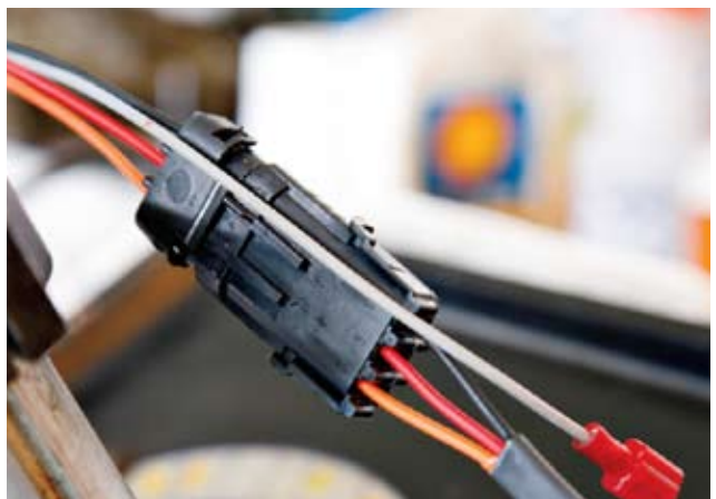
7 Connecting the MSD Pro-Billet distributor is as simple as connecting four wires. The red (switched 12V positive), orange (negative side of the coil), and black (ground) are grouped into one waterproof connector. The single gray wire is for the tach; it's also the wire used to program the internal rev limiter.
