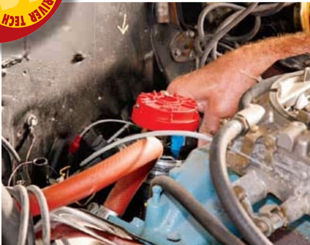
4 The MSD distributor slides in using the two marks we left on the firewall.
